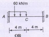
III. Draw the shear force and bending moment diagram by constituent deformation method. EI is constant.
