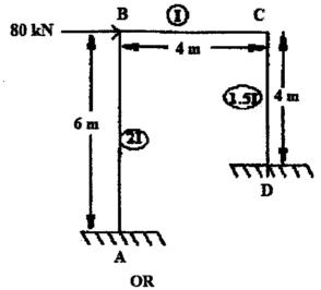
IX. Analysis the frame shown in figure by moment distribution method and draw the BMD. Assume EI is constant.
