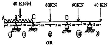
VII. Determine the support moments and draw the BMD for the continuous beam shown in figure.
